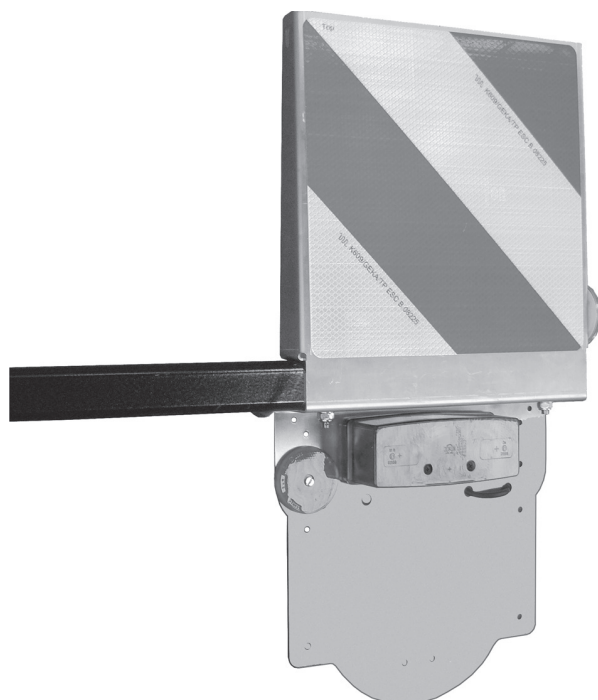
Fig. 50; Rear warning sign and lighting
