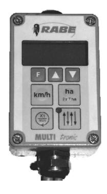
Operating instructions Seed drill monitor Multitronic II for Turbodrill L / XL ... A Turbodrill XL Combi-Speed ... A
